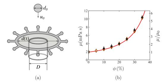
FIG. 1. (a) Schematic of the experimental setup. (b) Viscosity of a suspension of  $2a = 140 \ \mu m$  particles (black full circles) as a function of the volume fraction  $\phi$ . The red curve is given by Eq. (1), which allows us to obtain water-glycerol mixtures with equivalent effective viscosities (brown empty diamonds). All viscosity values are measured at T = 23 °C.
