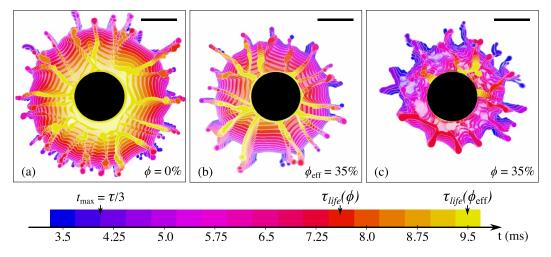
FIG. 7. Illustration of the retraction path: superposition of images during the retraction of the liquid sheet for (a) the carrier fluid, (b) the equivalent fluid ( $\phi_{eff} = 35\%$ ), and (c) a suspension of 140  $\mu$ m particles at  $\phi = 35\%$ . The first image (in blue) is 3.5 ms after impact, and the interval between images is 0.375 ms. Scale bars correspond to 5 mm.
