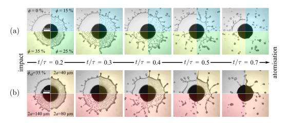
FIG. 3. Top view of the time evolution of the suspension sheet from the impact to the fragmentation in smaller droplets for (a) increasing volume fraction ( $\phi = 0\%$ , 15%, 25%, 35%, clockwise) of 140  $\mu$ m particles and (b) increasing diameter of particles (equivalent liquid, 2a = 40, 80, 140  $\mu$ m) at a volume fraction  $\phi = 35\%$ .
