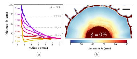
FIG. 2. (a) Radial evolution of the thickness of the liquid film for different times after impact from 2 to 8 ms. These curves were obtained with the carrier fluid (without particles). The dashed lines show the particle sizes for comparison. (b) Typical spatial distributions of the thickness at maximum spreading ( $t = \tau/3 = 4.2$  ms) for the carrier fluid. The correspondence between thickness and colors is indicated in the color bar. Scale bars are 2 mm.
